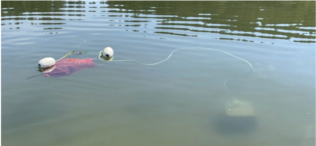
Figure 5.9 A BuDS setup showing the net bag of reproductive shoots clipped to the floating line at the buoy end. Credit: A. Spooner
