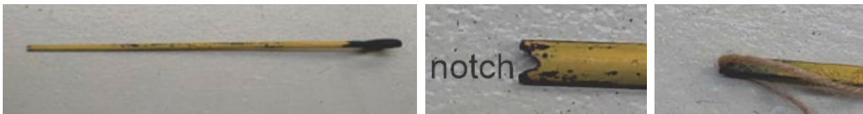
Figure 4.7 Threading tool made with a BBQ skewer. A notch at the end helps with threading.
